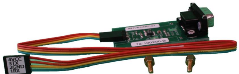
↖ RS-232-UART Level Shifter with cable
