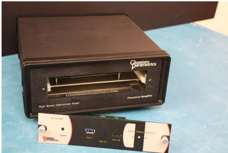
Figure 1 - HSIT with Connector Saver
