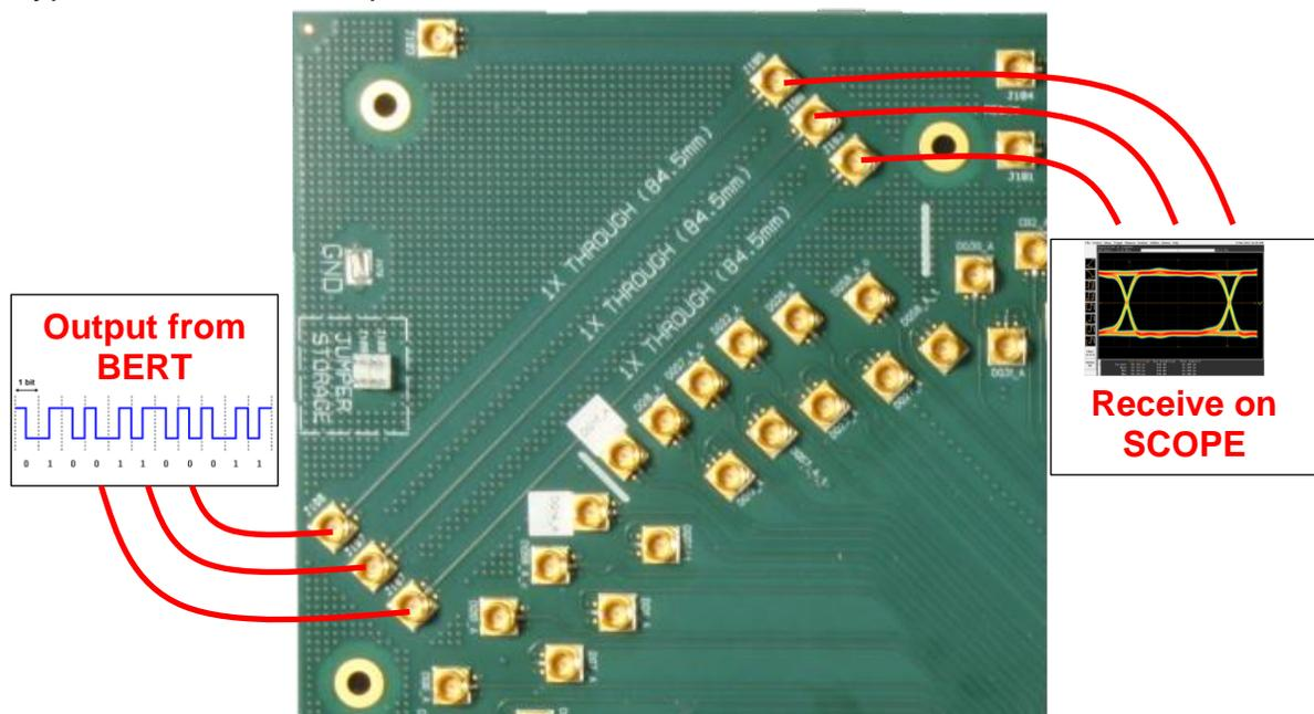
The 1X THRU trace is the same length as the traces from the DIMM connector to the SMP connectors. Therefore, this calibration structure allows the user to “view” the signal as observed at the DIMM connector location rather than at the SMP on the CTC2. This allows for better calibration of the signal from the BERT because the effects of losses on the CTC2 PCB can be accounted for. A more accurate measurement can then be made.
