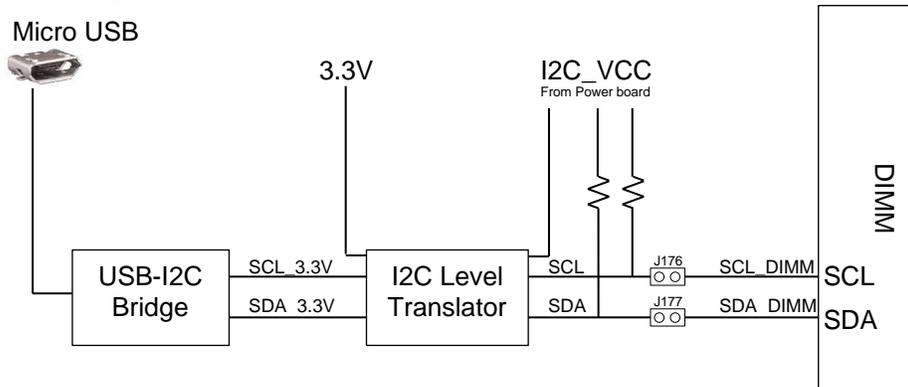
The CTC2 uses a Micro B USB connector to access the I2C/SMBus bus on the DDR5 socket. (SDA – Pin 5, SCL – Pin 4)
