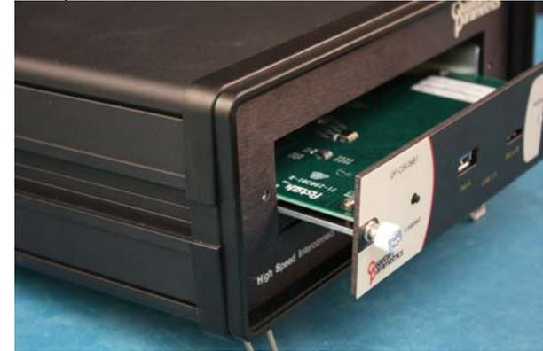
Figure 2—Connector Saver Module and HSIT device
