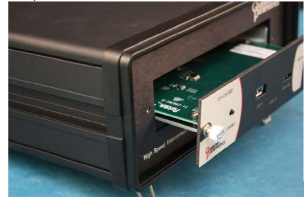
Figure 2—Connector Saver Module and HSIT device
