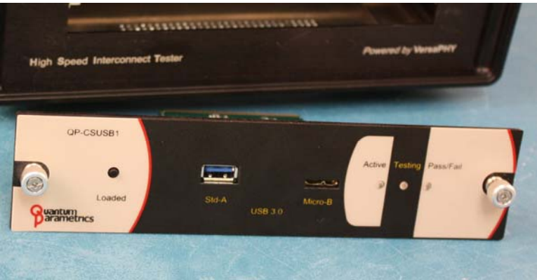
Figure 1—The HSIT USB 3.0 Connector Saver Module
