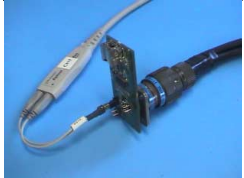
Figure 39 - C-1 Far End signal amplitude measurement.
