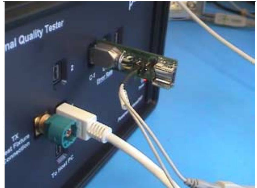
Figure 37 - C-1 Near End signal amplitude measurement.
