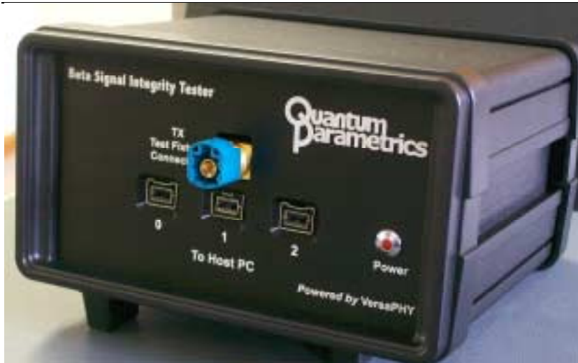
Figure 2 - Front Panel of Beta Signal Integrity Tester
