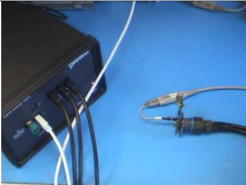
Figure 38 - SQT to 38999 Far End test fixture setup.
